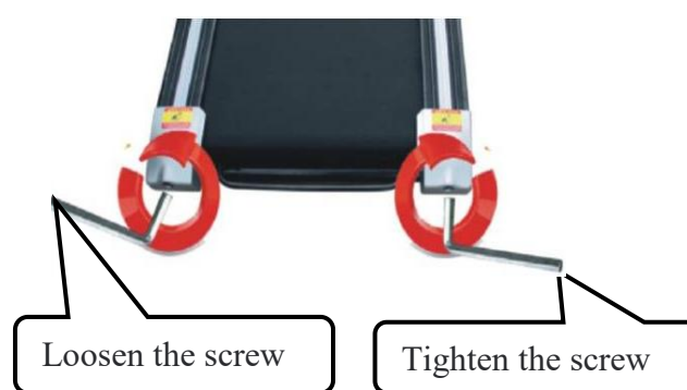
Picture B Adjustment Method for Right-sided Running Belt Deviation
